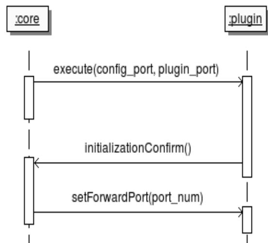
Fig. 7. Plug-in initialization sequence
