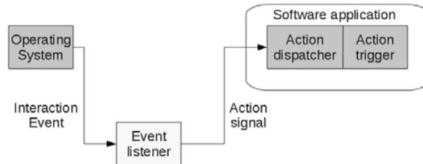
Fig. 5. Proposed action triggering
