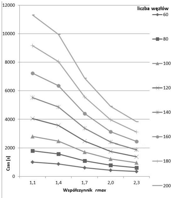
Fig. 4. The time at which the meshless algorithm achieved an analytical solution depending on the  $r_{max}$  coefficient and number of nodes
