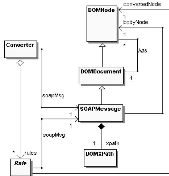
Fig. 6. Core classes of the Converter
