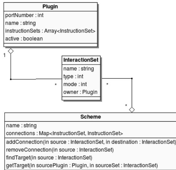
Fig. 9. Scheme structure
